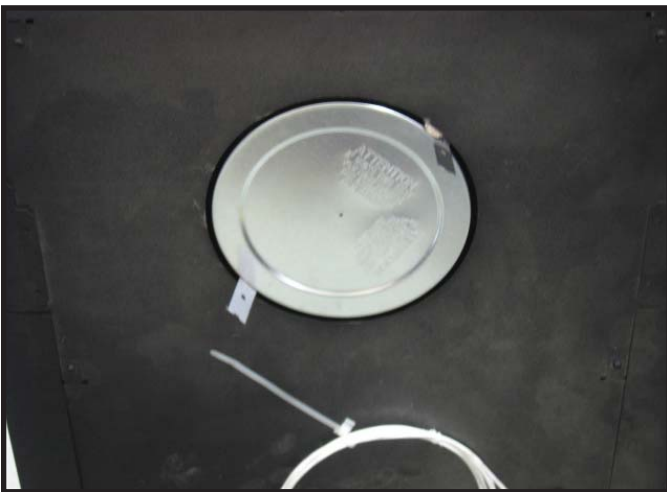
Figure 9.6 Remove the seal cap.
